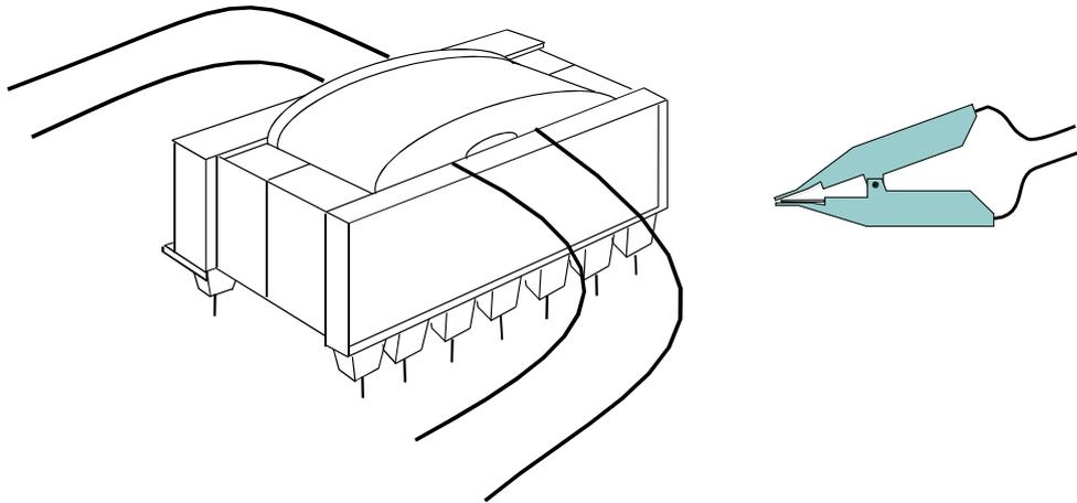
Kelvin connected alligator clips can be used to make connections to larger leads, shorter leads, foil leadouts or tags or screen on the top or side of the transformer. Screw one face of the clip down against the fixture plate for a permanent, easy-to-use connection.
