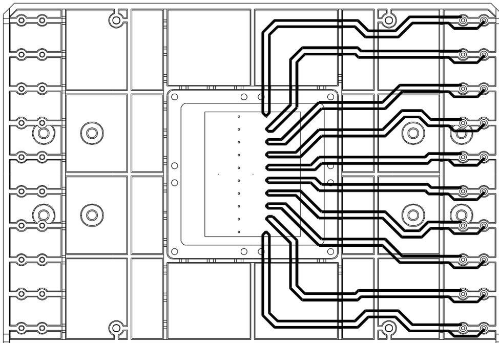
4 Start at the spring probe receptacle / Kelvin pin end and lay each wire neatly into the slots in the base plate walls.
